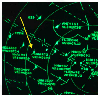
ATC radar with transponder on [2]
